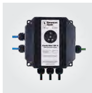
The Earth-Rite FIBC can be installed in Zoned / Classified combustible dust atmospheres. If gas and vapour atmospheres are present an Ex(d) / XP, Zone 1 / Class I, Div. 1 system may be specified.
