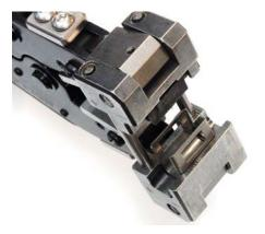
Insert the system cable into the metal bracket and turn it until it lies flat in the bracket. The negative pole (white marking) must be aligned toward the front of the pliers and correspond with the + and - imprints on the sides of the pliers.
