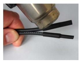
Compress shrink tube ends in the hot condition
