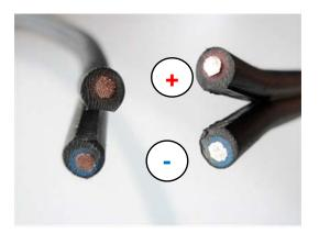
Open up the strands of the two system cables along a length of 5 cm
